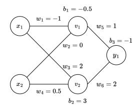
a) [4 points] Consider the simple neural network computing the function f as given above, with all nodes using the ReLU activation. You are given two datapoints  $d_1 = (1,3)$  and  $d_2 = (-2,0)$ . Biases are given explicitly as values at the nodes. What is the output of the network for these two values?
