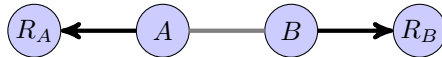
Figure 10.21: The exposed terminal problem: senders A and B could send to their respective recipients R_A and R_B simultaneously, but believe it would cause collisions due to carrier sensing.
