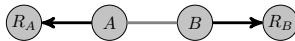
Figure 10.21: The exposed terminal problem: senders A and B could send to their respective recipients R_A and R_B simultaneously, but believe it would cause collisions due to carrier sensing.
