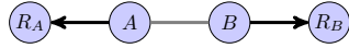
Figure 5.41: The exposed terminal problem: senders A and B could send to their respective recipients R_A and R_B simultaneously, but believe it would cause collisions due to carrier sensing.
