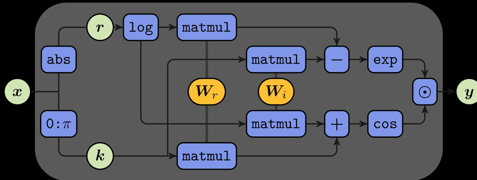
NaiveNPU diagram, with input  $x$  and output  $y$ . Vectors in green, trainables in orange, functions in blue
