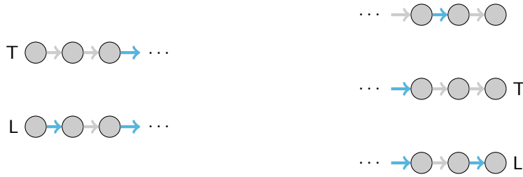
Figure 12.30: The possible constellations at the beginning of a path on the left: the start node can be tight (T) or loose (L). In the former case, the first edge is rounded down, in the latter it is rounded up. Starting from the second edge with a drop, there is a perfect alternation until before the end of the path. The possible constellations at the end of a path: If the path has even length, the last edge will be rounded down (in accordance with the perfect alternation) regardless of whether the end node is loose or tight. If the path has odd length, the last edge will only be rounded up if the end node is loose; otherwise, the last edge will be rounded down.
