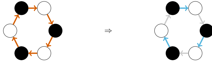
Figure 6.21: A perfect rounding of a 2-colored cycle with a given orientation of the cycle. An edge is rounded up (blue) if it leads from a node with color 1 (black) to a node with color 2 (white) and rounded down otherwise (grey).
