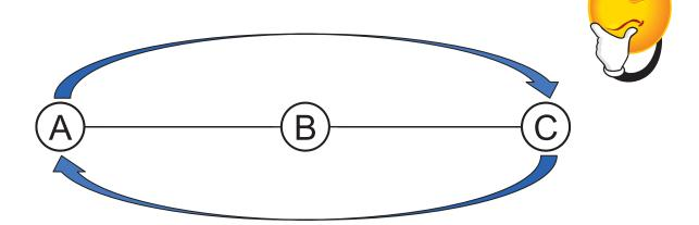
Traditionally, intermediate nodes in networks just forward data. Network coding deviates from this paradigm, in the sense that intermediate nodes are allowed to process data before forwarding!
