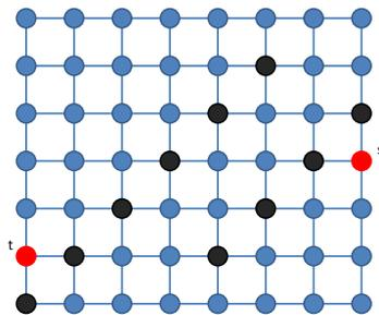
Figure 1: Strategy for  $w \approx h$  with faulty nodes marked as black. The longest shortest path leads from  $t$  to  $s$
