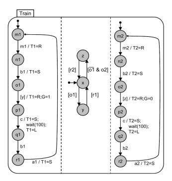
• The trains start at their states m1 and m2. When m1 (m2) is pressed, then train 1 (2) moves to the right in n1 (n2), until it reaches the switch, where it stops in state o1 (o2).
