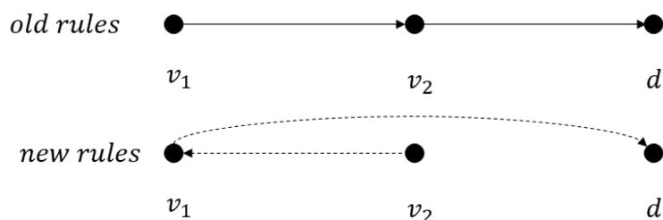
Figure 1: Simple example: In the old rules,  $v_1$  forwards to  $d$  via  $v_2$ , and  $v_2$  is directly connected to  $d$ . In the new rules,  $v_2$  forwards to  $d$  via  $v_1$ , and  $v_1$  is directly connected to  $d$ . The node  $v_2$  may not migrate in a first update step, because that would induce a potential loop between  $v_1$  and  $v_2$ !
