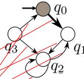
As a Boolean function:  $\psi_S(q, q') = \overline{x_0}' \cdot (x_0 \cdot (x_1 + x_1') + x_1 \cdot x_1') + \overline{x_0} \cdot x_0' \cdot \overline{x_1}'$
