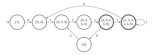
It can easily be seen, that first the states  $\{4\}$ ,  $\{2,4\}$  and then the states  $\{2,3,4,5,6\}$ ,  $\{1,2,3,4,5,6\}$  can be merged and hence, the automaton can be reduced to the one shown in the next figure.
