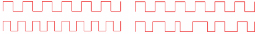
Figure 7.8: Drift (left) and Jitter (right). On top is a square wave, the wall-clock time t^* .
