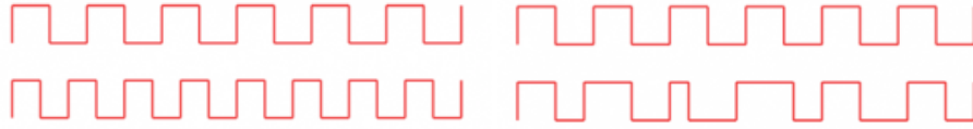
Figure 20.8: Drift (left) and Jitter (right). On top is a square wave, the wall-clock time t .
