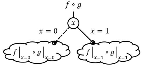
Boolean functions can be converted to BDDs step by step using APPLY.
