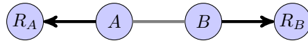
Figure 5.41: The exposed terminal problem: senders A and B could send to their respective recipients R_A and R_B simultaneously, but believe it would cause collisions due to carrier sensing.
