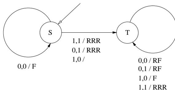
and  $T$  (Track). The robot starts in the Seek state, not knowing anything about its position. The goal of the Seek state is to find a wall. Once a wall is found, the tracking works by following the *wall to the rear-right* condition. That is, there is always a piece of wall to the right of the robot, or diagonally to the rear-right, or both.
